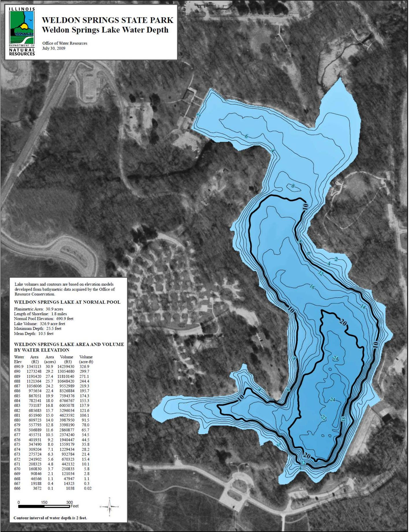
Lake volumes and contours are based on elevation models developed from bathymetric data acquired by the Office of Resource Conservation.
